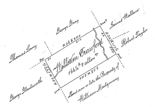
The above is a Draught or representation of part of a Tract of land which contained Three hundred and thirty two acres and an half of an acre and Allowance of Six p! lent. Dituate on the North Side of Conemaghi on a branch of Black legs creek, which Tract was Durvey de to Andrew Dimpson on the 22 May 1771 by Order of the 3 April 1769. No 2699
